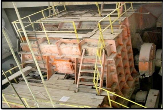
**Gambar 1.** *Hammer Crusher*
